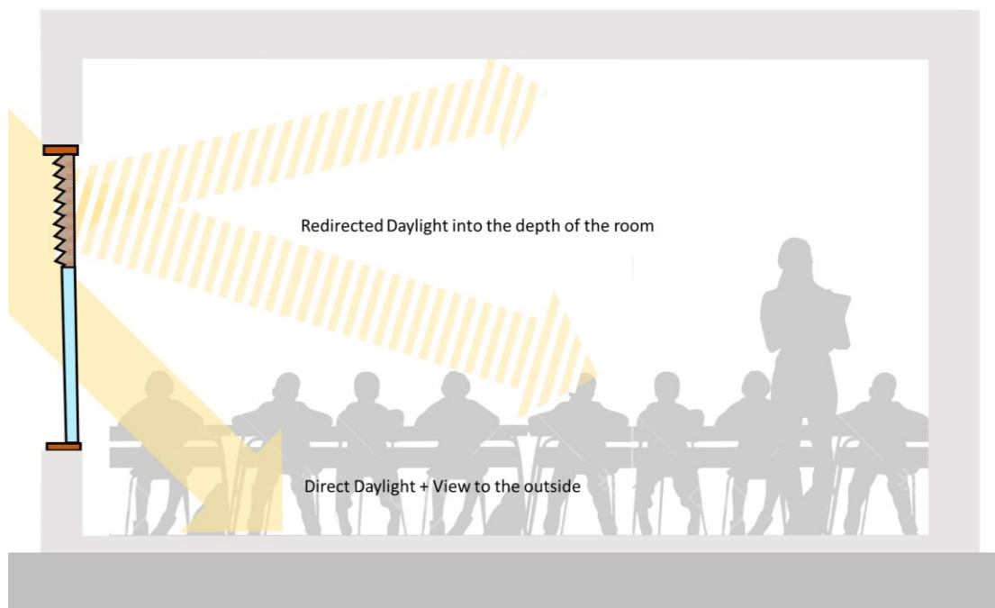
FIGURE 63 POSSIBLE SETUP FOR THE CFS IN SPACE WITH VIEW TO THE OUTSIDE NEEDED
